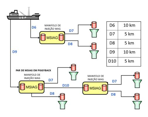
NOTE: The umbilical lengths (Dn) are just a reference. The SUPPLIER shall request from the CONTRACTOR the lengths to be used for the HPU's dimensioning.
