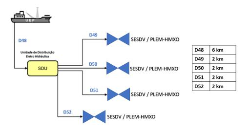
NOTE: The umbilical lengths (Dn) are just a reference. The SUPPLIER shall request from the CONTRACTOR the lengths to be used for the HPU's dimensioning.
